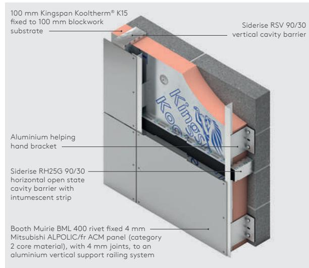
Figure 1: FR ACM panel & Masonry Blockwork
