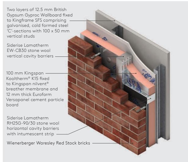
Figure 2: Brickwork Facing & Kingspan Kingframe SFS
