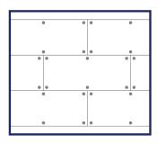
On metal decks the long edges should be laid at right angles to the corrugations. All board joints should be fully supported by the deck.
